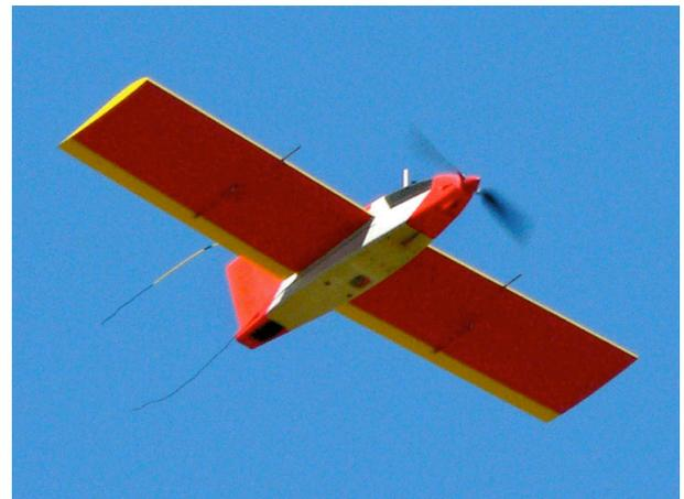
Figure 2 Experimental UAV with down and forward looking camera
