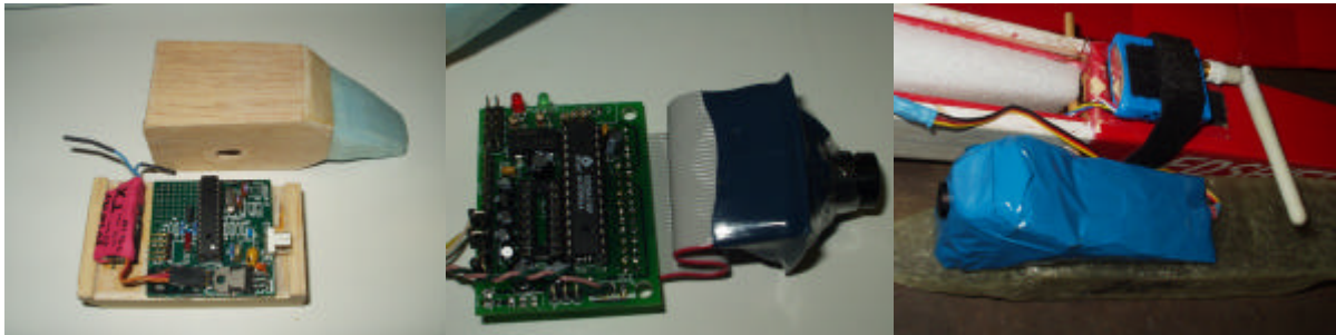
Fig. 3 Airborne equipment, left to right, microcontroller with data telemetry radio, OV6620 camera with CMUCam image processor, analog video camera and video telemetry radio
